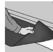
**EN:** If the base is of concrete a DPC must be placed under the whole length of the threshold.
