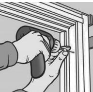
**EN:** Place exactly fitting blocks where the windows fixing holes are positioned, and fix with screws where the predrilled holes are positioned in the frame.
