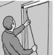
**EN:** Side jambs must be adjusted to be vertical and in plane and all diagonals
