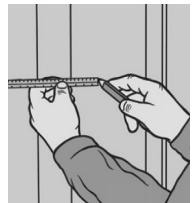
**EN:** Decide and mark the position of the frame in relation to the inner and outer wall.
